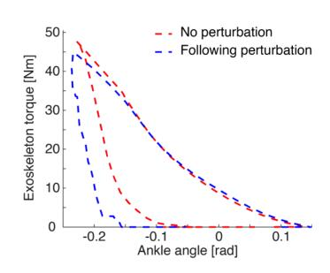
Modulation of ankle angle-torque profile to assist in balance recovery
