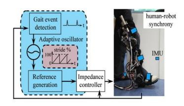
Gait-event-based synchronization method using an adaptive oscillator.
